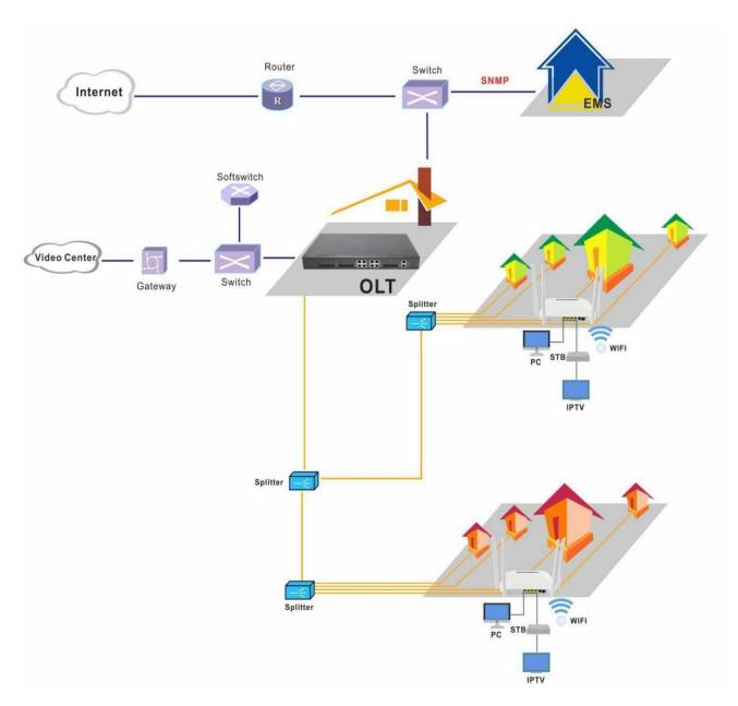
Figure: NTPL-XPON1G3FEACV Application Diagram
